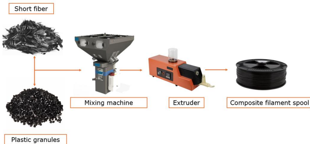
Fig. 2. Processing of FDM filament with short fibers by mixing and extrusion
